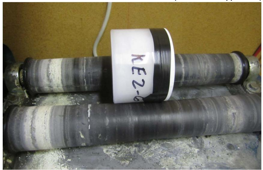
The Mill was Opened After 10 minutes just to Show the Bubbles and Viscosity. Pll Sometimes also uses Teflon Pipe Tape on the Jar Threads if Leaking is a Problem.
