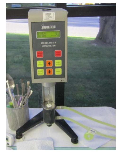
Close Up of the Small Sample Adapter SC4 21/13. Slurry Viscosity Measured ~140 cps at 20 rpm (18 1/sec)
