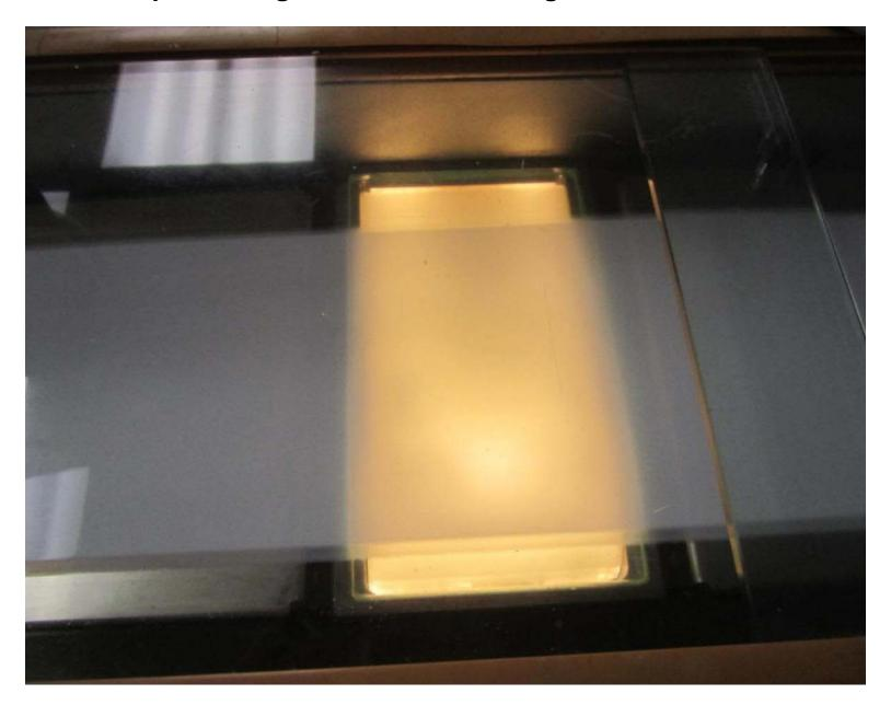
Zone Temperatures Depend On Tape Thickness, Caster Type and Desired Casting Speed (Typical Lab Settings Provided). Adequate Air Flow Depends on Caster.
