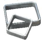
with a depth or a clearance of one mil will lay down a film approximately 1/2 mil thick. A latex film will shrink considerably more, so paths of greater depths are required in order to obtain a dry film thick enough to check flexibility and toughness.
