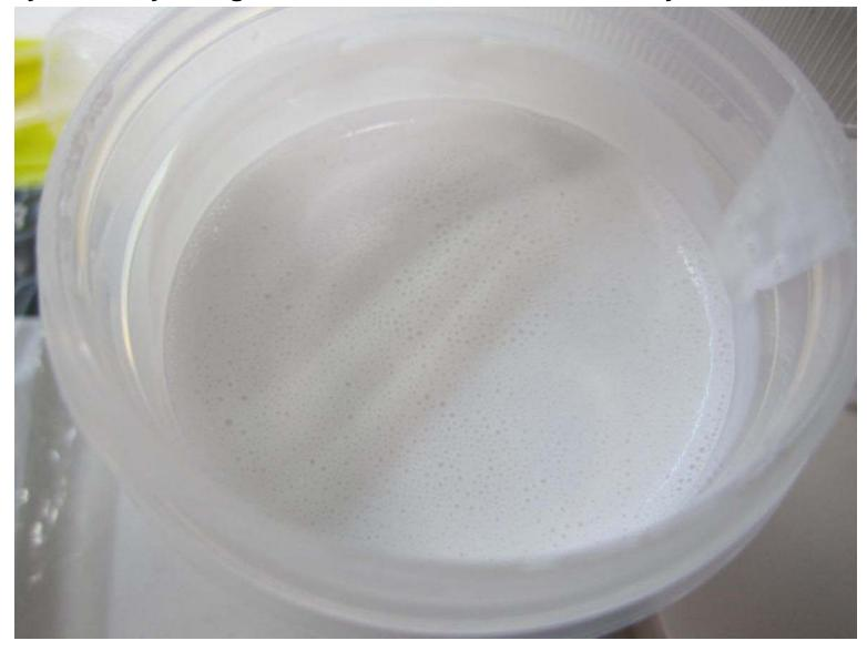
The pH of the Slurry was Measured at 7.0. A Normal Range for this Powder is About 6.5 to 8.0 but for Other Ceramics the pH is Normally Higher. If the pH is less than about 6.5 the Binder Can be Unstable and Needs Adjustment
