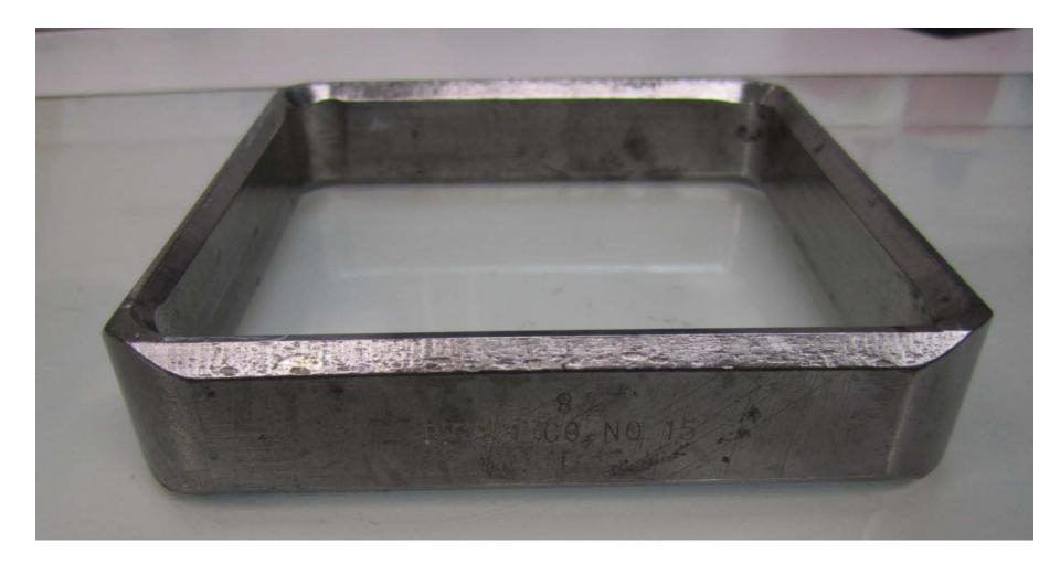
SiPET Rolled Out on Flat Glass Surface and Slurry Poured Into Hand Doctor Blade. This method will create thin spots as a result of air trapped under the siPET and glass but otherwise acceptable results. Tape can be left flat to air dry or hung from a vertical surface.
