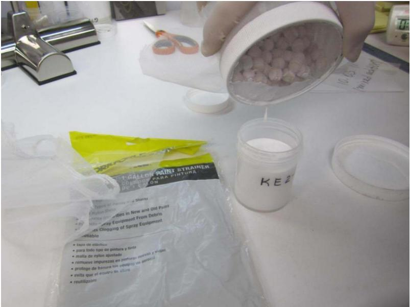
Close Up of Minor Foam on Freshly Drained Slurry. Easiest Way to Deair is to Allow Slurry to Sit Without Stirring for at Least Several Hours. For Other Powders if Slurry Viscosity is High or Needs to be Cast Immediately use Vacuum Deairing
